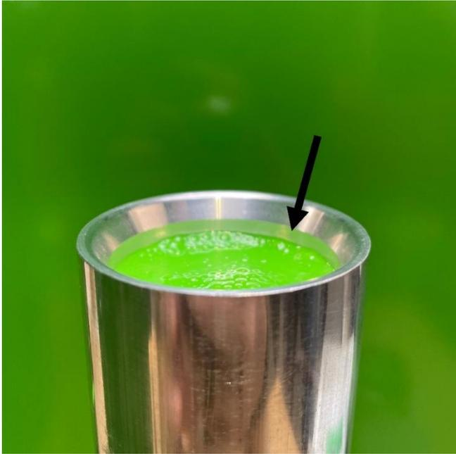
Carefully pour 100 ml of paint into the filling cylinder, just below the indicated mark.
